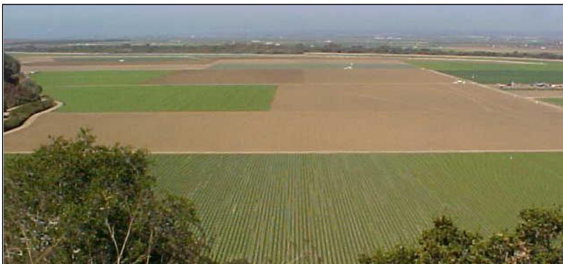
Salinas Valley agricultural lands near Castroville, California, 2003. The rectangular grid pattern of Public Land Survey System is clearly evident in this photo. Photo: Neal McLain.
