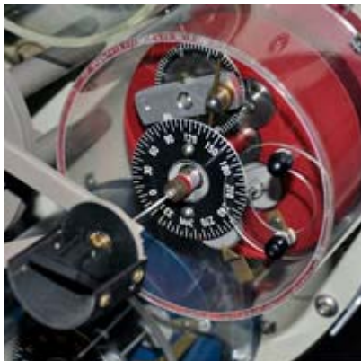
Left: Analog computer for tracking the motion of Mars.
