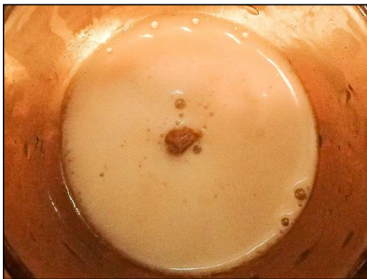
Acid test: 5% HCl was added to the specimen. Foaming occurred immediately but no large bubbles occurred.
