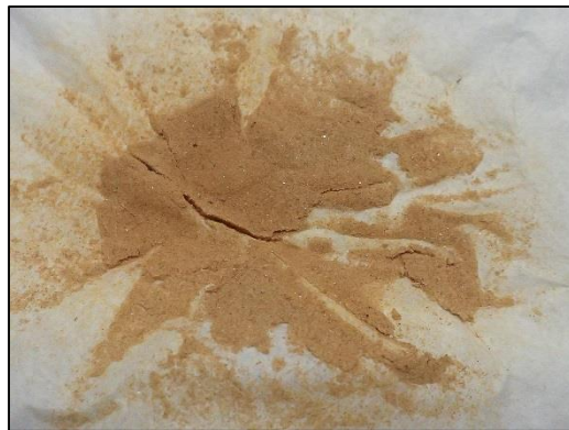
Post-acid test: specimen was filtered, rinsed and allowed to dry. Specimen residue weighed 2 g. Considerable sand remained after the acid test was done.
