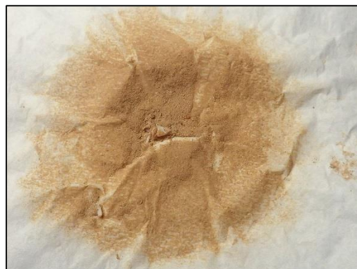
Post-acid test: specimen was filtered, rinsed and allowed to dry. Specimen residue weighed 1 g. A small amount of sand remained.
