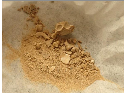
Tested specimen: 4 g; specimen was coarsely pulverized prior to testing. Pulverized specimen has appearance of fine sand.
